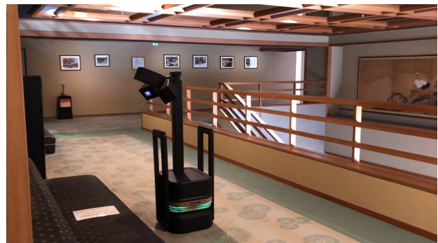
"UV Light irradiation package next generation concept model" that performs UV irradiation in the hotel.
